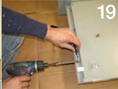
James installs the hardware, securing the tailgate strap fitting to the inside edge of the tailgate.
