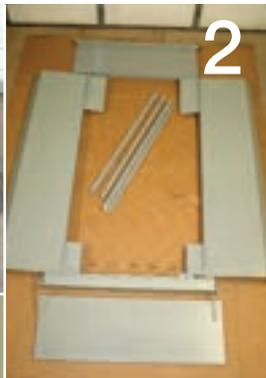
*Before beginning we laid out all of the parts included in the Pro's Pick bed kit. A bulkhead panel, two bed sides, three bed frame cross members, one rear cross member, and a smoothie tailgate were set up to start the job. Tools needed included 1/8, 5/16, 11/32, and 17/32-inch drill bits; a drill; 9/16, 1/2 and 7/16-inch wrenches; a tape measure; and a felt tipped marker.*
