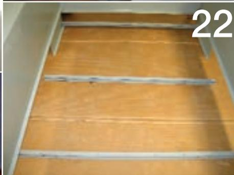
The Pro's Pick X-members should all be marked with a tag to determine their position. It's never a bad idea to mark them with a felt tipped pen so you have a constant visual. Exact placement of the X-members in our case is not a definite at the moment since we will be building a custom, raised bed floor to accommodate our deeply notched frame. If you are installing on a stock F-100 chassis, follow the Pro's Pick instructions.
