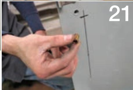
This threaded insert will be installed to secure the bedside end of the strap in position.
